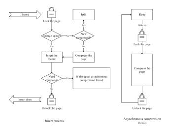
Fig. 5. Asynchronous Compression
