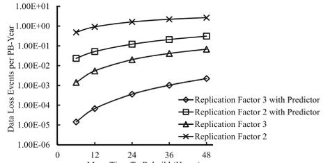
Fig. 8. The change of systems reliability according to the rebuild time.
