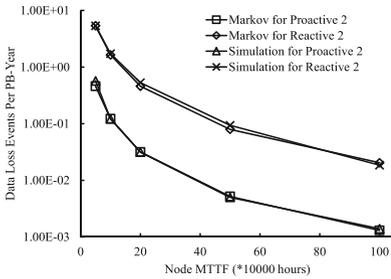
**Fig. 5.** The change of the reliability of systems with replication factor 2 according to the node reliability.
