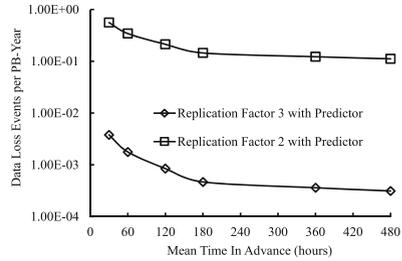
**Fig. 10.** The change of proactive systems reliability according to the mean time in advance of predictors.
