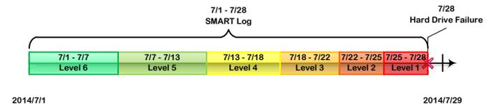
Fig. 2. An example of health degree settings. The health status of hard drive is splitted into 6 health degree levels. The closer to the time point when the hard drive break down, the lower the health degree is.
