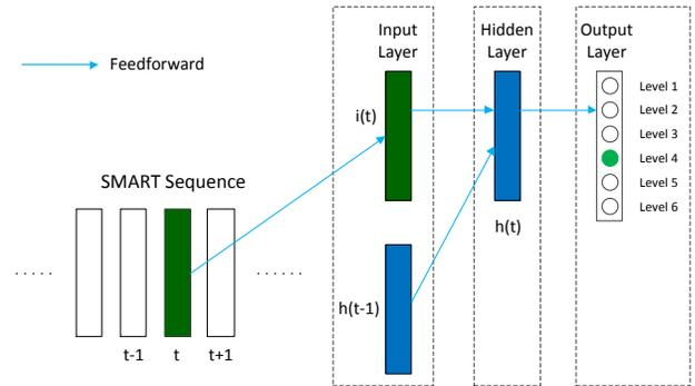
Fig. 3. The testing process of the RNN-based health degree assessment model. The inputs are the sequential SMART records. The outputs of the hidden state are computed based on the  $(t - 1)$ -th SMART sample and are used as the inputs, together with the  $t$ -th SMART sample, to assess the health degree of disk drive at time  $t$ .
