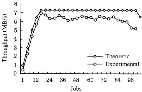
Fig. 5 Comparison of the theoretic and experimental throughput.
